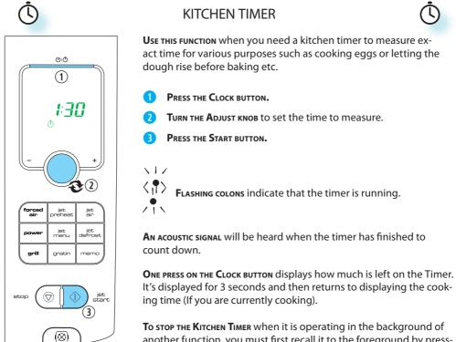
To STOP THE KITCHEN TIMER when it is operating in the background of another function, you must first recall it to the foreground by pressing the Clock button and then stop it by pressing the Stop button.
